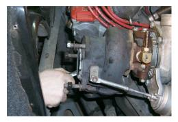
NOTE: A QUALITY wrench must be used on the nuts. DO NOT use a Craftsman wrench on the nuts, or any other "inexpensive" openended wrench. I have seen the wrench head flex during attempted removal.
