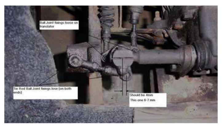
4. If necessary, adjust the length of the two cables at their rear end ball joints so that they can be connected to the translator without preload. Note that both gearchange cables are identical and that the right hand cable at the gearlever end is fitted to the left hand side of the gearbox end. As a check, move the gear lever across the gate from right to left and observe cable movement at the rear end. The cable that moves forward is fitted to the left hand side at the gearbox.
