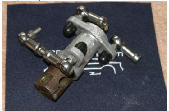
• The job is now nearly done. Check that all gears can be selected. If there are any problems selecting reverse or 5<sup>th</sup> gear then the chances are you will need to make a small adjustment to the tie rod length. The alignment directions provide by Lotus are attached to help with any fine tuning required.
