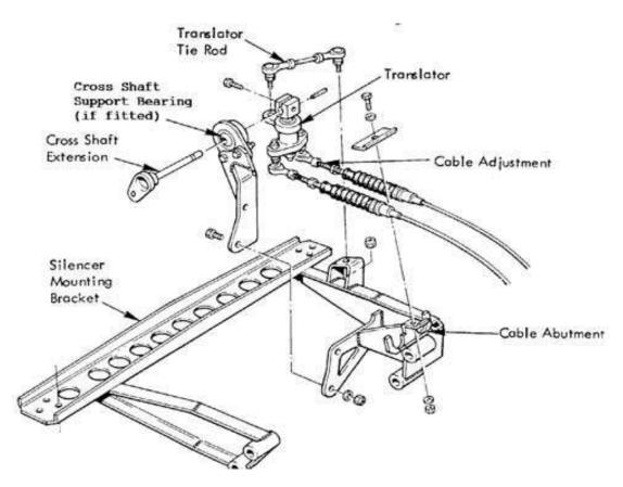
The translator consists of two parts: a swivel 'tree' and a pivot pin, the pivot pin hangs from a splined clamp which is secured to the cross shaft extension. The swivel tree which pivots on this pin via two ball bearing races, has two diametrically opposed arms at its lower end and a single arm disposed at 90° to the others, at its top end.
