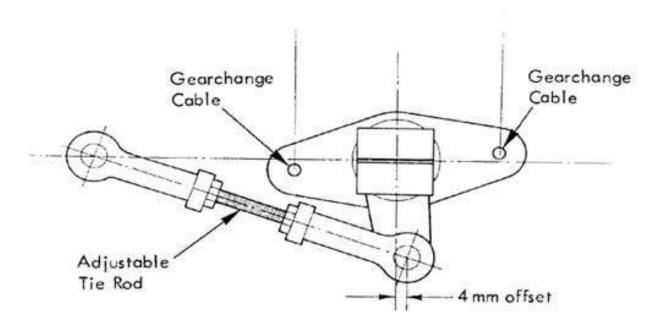
3. The gearchange lever is independently spring loaded to the 3rd/4th gear plane. With the aid of an assistant, hold the gear lever leaning backwards approximately 7.5° in this crossgate plane.
