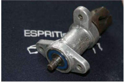
• With the central shaft in place, slip the large dia washer over the threaded end of the shaft, followed by the original thick washer. The new large dia washer helps keep muck away from the bearings for longer. Finally fix the new nylock M8 nut onto the shaft and tighten until its snug against the washer. The central shaft should now rotate freely on the new bearings without any slop or rough motion.
