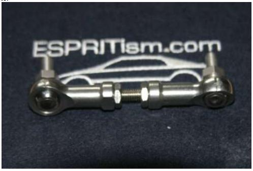
• Now fit the new tie rod assembly to the translator body and exhaust mounting bracket. Use the provided M6 nylock nuts to fix the rod ends in place.
