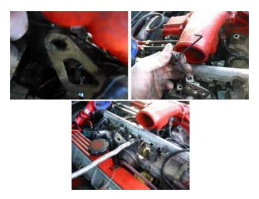
You can then remove the connection and the rod will be free. You can see the allen key in the grub in the middle picture above.
