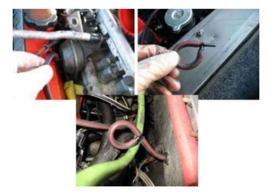
Now you need to remove the vacuum pipe from the capsule and block it off. We like to use a t-piece to feed the pipe back on it's self, We cut the pipe closer to the bodywork to keep it tidy. You can push a ball bearing into the pipe or a screw, but you must block off the pipe.
