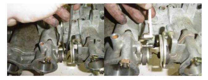
LEA has removed the quadrant successfully, you look closely of its base, the quadrant uses a clip which can be removed with a screwdriver by taking the clip away from the assembly the quadrant can be now slide from the little rod holding it, see photos below. This removal was done after we removed the inlet manifold so it was easier to access however this can be done by removing the plenum nozzle.
