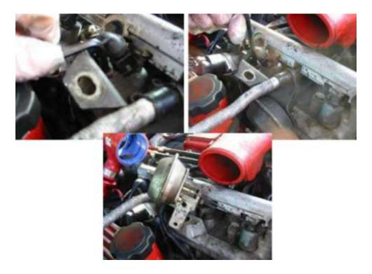
Two allen head bolts hold on the bracket, which is actually one of the chargecooler mountings. Once this is removed you can pull it and the capsule out.
