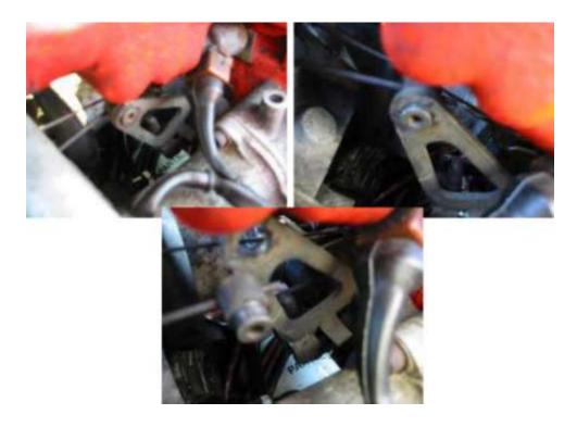
To remove the rod from the triangular piece (quadrant) just use an allen key to unscrew the grub holding the rod tight
