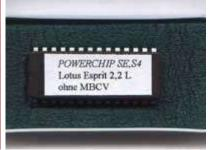
Your new chip is supplied with a chip holder. This is what will replace the chip, this will then allow you to change the chips. Now if you're happy to do the soldering yourself, take a pair of scissors and carefully cut the 28 connectors holding the chip in. You can then solder the holder into the space where the chips just been removed from.
