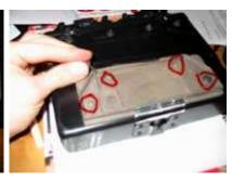
Once the holder has been soldered in place, all you now need to do is attach the chip to the holder and replace the blue cover. The cover may not fit as the holder had been soldered a little to high on the board. This isn't a problem as you can leave it off. You can now reattach the ECU to the Esprit. Once everything is replaced, you can now start your Esprit and test your chip.
