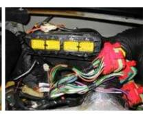
You'll see the ECU as soon as the covers removed. It's the black box with four large red connectors attached to it. You now need to remove the wires from the ECU. Push down top and bottom of each connector and pull them off. Mine were a little stiff and needed pushing down quite hard. (If you don't want to disconnect the ECU, you can turn it over and remover the chip while it's still attached). Remember to note which connector is attached in which order. This will help when replacing the ECU.
