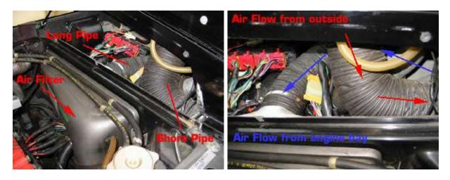
You'll see two pipes. One is short and goes from the outside air intake (behind the rear quarter light), into the engine bay. The second pipe is much longer (see picture below) and goes from the engine bay tube into the air box. You can see the pipes above, with the short pipe dropping down and running off to the right and the longer pipe running from the far left, passed the short pipe and off to the far right.
