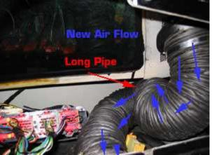
You now have two pipes off the car. To complete the conversion you have two options. You can use the long pip to connect from the outside intake straight to the airbox. This allows you to put the system back to it's original design. But this also leaves you with a long pipe going from the intake to the airbox. Effectively slowing down the air flow to the air box.
