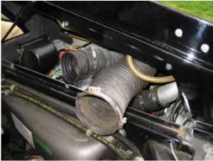
Once the jubilee clips have been loosen enough. You can pull the pipes off the four connections. Be careful not to disrupt anything else as there are other pipes and electrically connection
