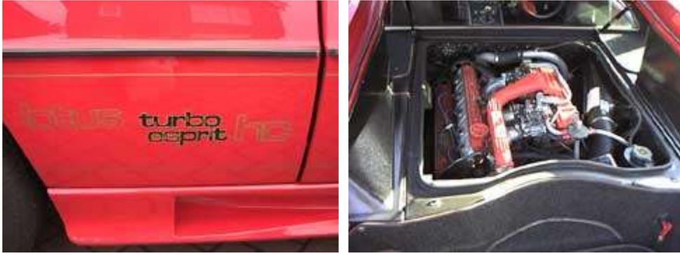
Mahle-forged pistons brought the increase in ratio from 7.5:1 to 8:1; Nikasil process for the liners was specified once more. Lotus rather reluctantly joined the European low-lead petrol age stating: 'The new Lotus turbo engine can be safely operated on unleaded fuel (minimum 95 RON). We recommend 4 star (98 RON) for maximum engine durability.' In other words, 'don't call us if it pinks a piston to death . . .'
