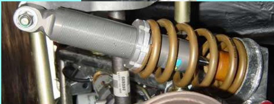
The suspension is now adjustable in height and made by eibach who are a well respected suspension manufacturer. These can be easily fitted to all V8's. Part numbers :
