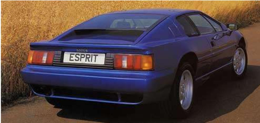
The new Esprit S features a 228bhp Lotus engine with multi-point fuel injection and catalytic convertor fitted as standard. Running on unleaded fuel, the Esprit S can achieve 155mph where driving conditions and regulations permit. An anti-lock power brake system is now standard equipment for all 1991 Esprits.
