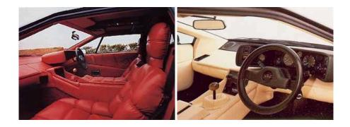
Cockpit changes have been made, including an instrument panel which now boasts a turbo boost gauge and speedometer running up to 170mph. Air conditioning controls are now situated in a centre console panel and all swithgear is backlit when main and side lights are illuminated. The seats have revised foam foundations and with new head restraints.
