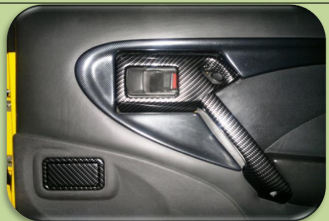
Handle, door interior grab, A082U6248F A082U6249F Cover, interior release handle, A082U6252F A082U6251F
